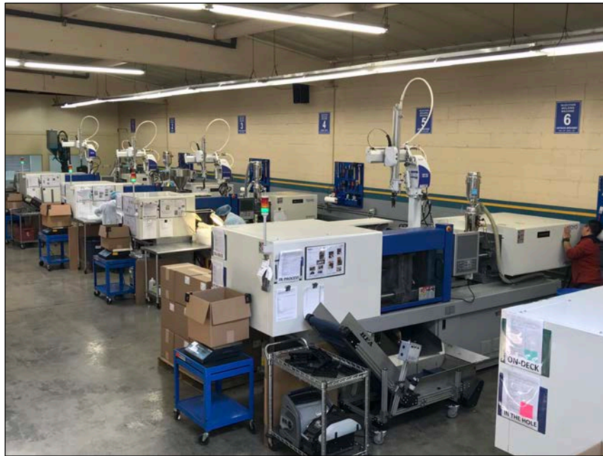
Precision Molded Plastics Inc. of Upland, Calif., has 14 presses, including nine efficient electrics and five hydraulics.
